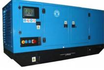
Prime Power (ISO 8528) ratings are suitable for continuous electrical power (at variable load) in lieu of mains power. There are no limitations to the annual hours of operation. Average 24 hr usage should not exceed 80% of the prime power. Models can supply 10% overload power for 1 hr in every 12 hr period.
